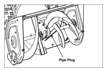
Figure 5. Checking Auger Gear Case Lubrication
